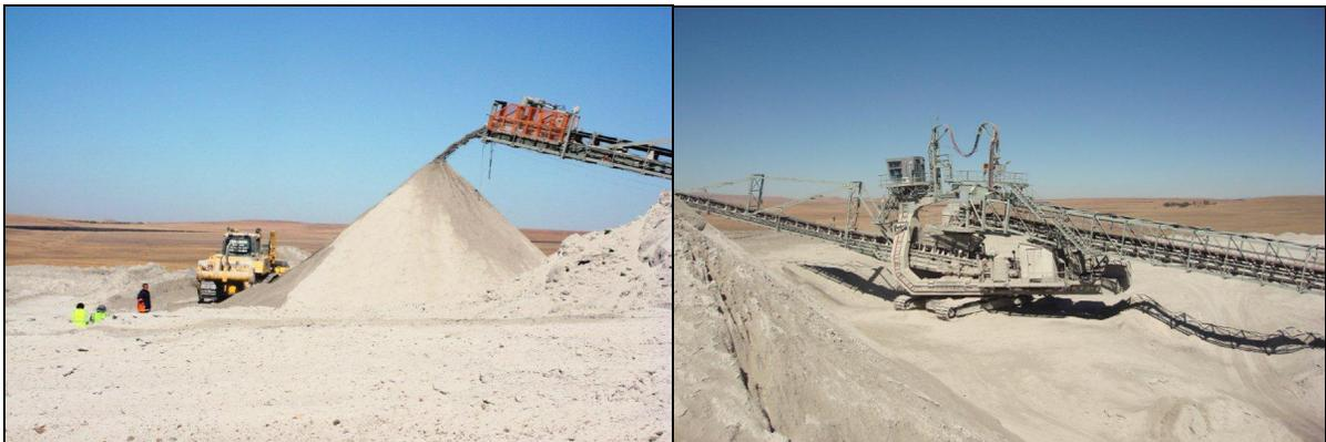
**Figure 1:** Stacker being used to dispose of ash at the Tutuka Power Station
